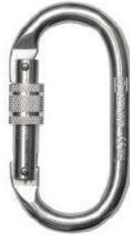
AZ 011 SCREW SNAP HOOK EN 362 Ref.: AZ 011 Weight: 180 g Dimensions: 108 x 60 mm ZINC PLATED STEEL
